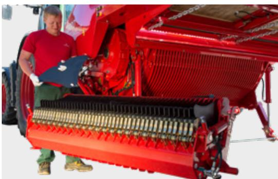
The knife retention springs and rollers on the individual knife protection system are swung safely out of the way. This greatly reduces the contamination of the knife holders. The chopping system can be pivoted out directly from the tractor seat to clear any blockages.
