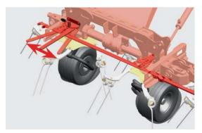
Actively setting the wheels at an angle causes the tedder to run diagonally so the forage is directed onto the mown area. Neighbouring crops remain untouched. Because the wheels can be set to the left or right, fenceline tedding can be activated in any driving direction.
