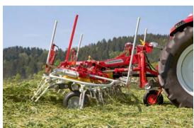
Ground tracking and forage protection are the key objectives of HIT rotary tedders. An optional jockey wheel on the pivoting headstock tracks the ground immediately in front of the tine path and responds to each undulation. The result: Clean forage, lower raw ash content and improved livestock health.
