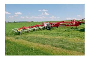
The trailed HIT T tedders with 10 or 12 rotors are designed for high output tedding. To meet the requirement of wider working widths and still provide the best possible ground tracking, the rotor units are linked together by individual hinge points. Combined with the chassis wheels guiding the rotors, HIT T tedders guarantee a perfect operation even at higher working speeds.
