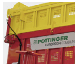
Hydraulic automatic loading flap
