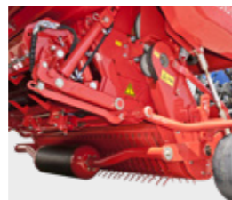
Additional tracking roller for pick-up
