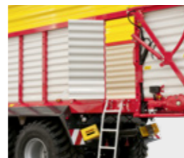
Access door with ladder
