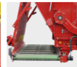
Cross conveyor belt
