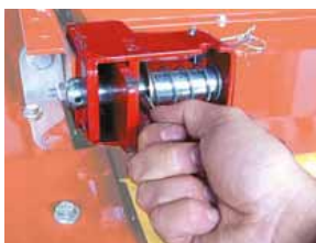
Quick-change pins for conditioner
