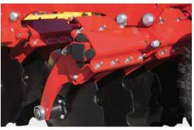
A uniform surface finish with the best mixing performance meets farmer's and contractor's expectations in the field. To achieve this, PÖTTINGER has optimised the geometry, size, mounting angle and penetration angle of the discs. The result: Low draft, perfect ground penetration, best tilth and mixing effect.
