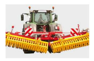
The large folding disc harrows have been developed for high output stubble cultivation and general seedbed preparation.
