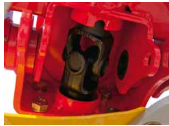
Permanently lubricated single and double joints
