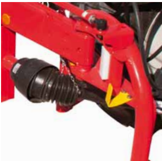
Steering angle indicator on the pipe bracket
