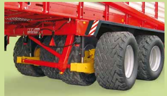
8-wheel chassis – perfect soil protection up to 22 sh t / 20 t total weight
