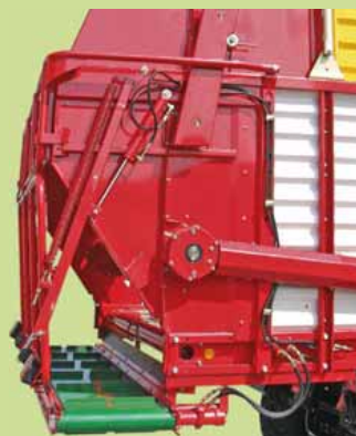
Hydraulic cross conveyor belt
