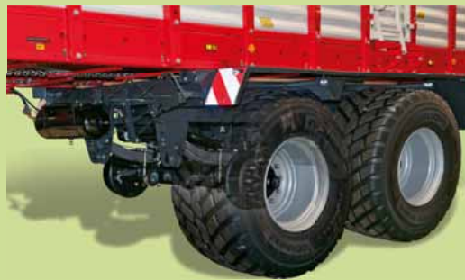
Parabolic spring chassis for up to 22 sh t / 20 t permissible laden weight
