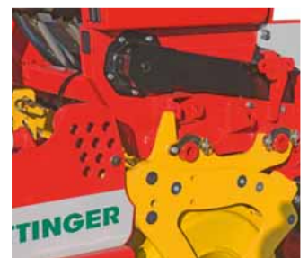
Attach retention bars to secure seed drill
