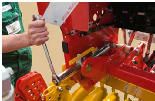
Central depth adjustment – easily accessible
