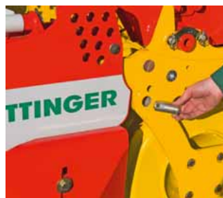
Remove fixing pins on rear roller for Parallelogram guidance
