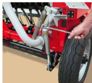
Central coulter pressure adjustment
