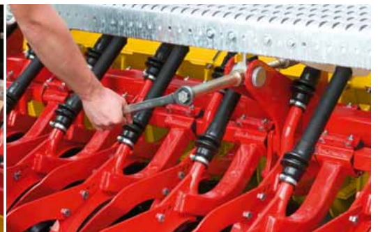
Central coulters pressure adjustment
