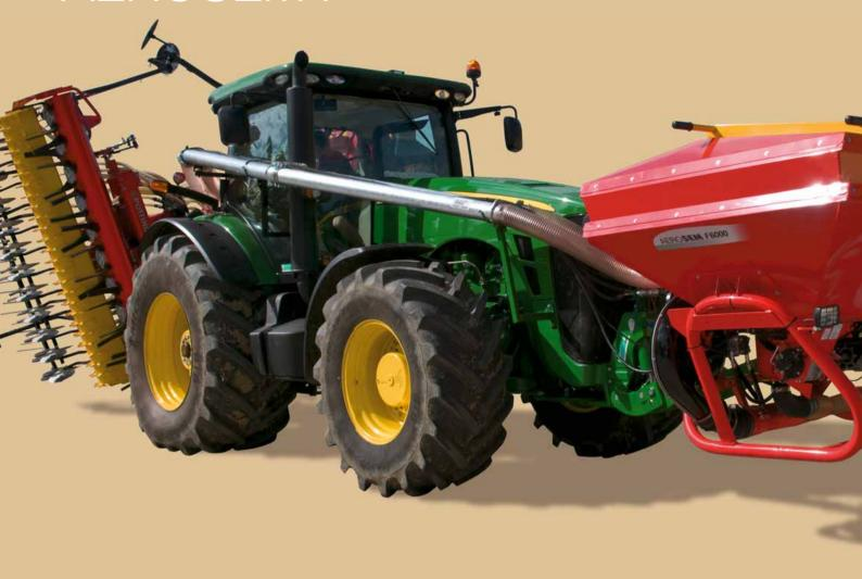
On pneumatic seed drills with wide working widths rear-mounted machines often exceed the axle load limits of the tractor. Steering becomes very difficult as a result. With the front tank version the hopper acts as ballast on the front axle. Reduced pressure on the ground and safe travel across slopes speak for the AEROSEM F from Pöttinger.
