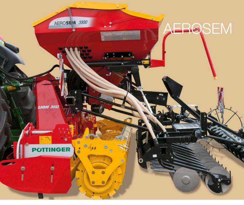
ORegardless of whether you are operating on light soil, heavy soil, dry soil or damp soil – the best possible placement of the seed is the key to a successful harvest. Different shapes of coulter with a gang spacing of 14' / 350 mm prevent clogging even when operating in harvest trash.
