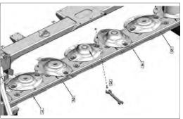
Reverse the three screws in the centre bearing.
