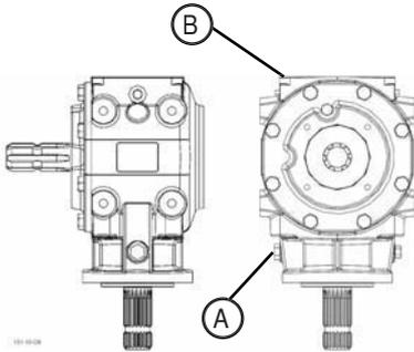
**Lubricate cross-feeding auger
