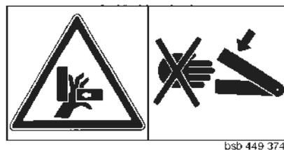
Never reach into the crushing danger area as long as parts may move.
