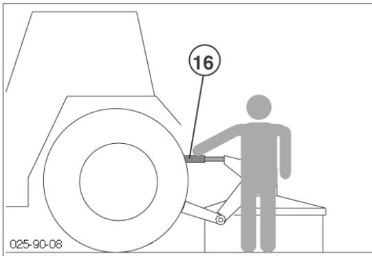
2. For mowing, slowly engage the p.t.o. shaft away from the crop and bring the mower rotor up to full speed.
