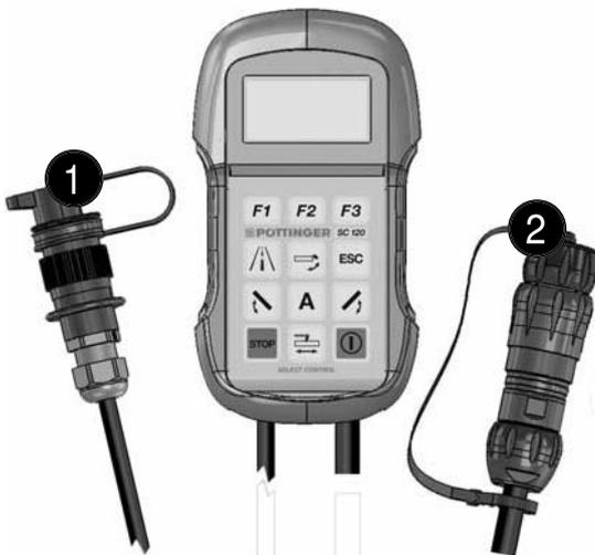
Position the Select Control terminal so that it is easily visible in the tractor cab. (There is a magnet on the rear for attaching the terminal.)
