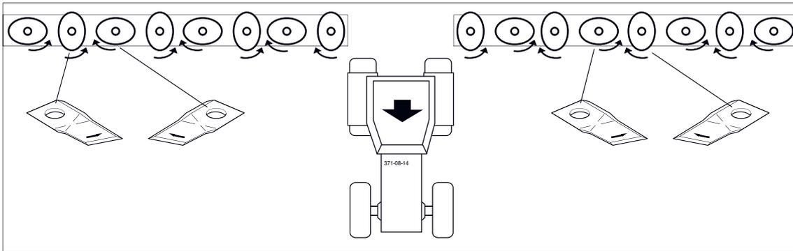
Checking wear on mowing blade holders
