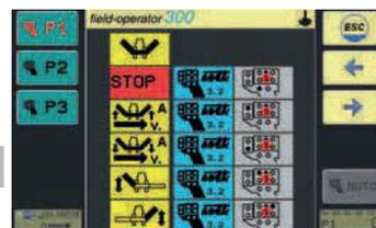
**Important:** The number on the joystick symbol (1/2/3) shows the level selected for the function!
