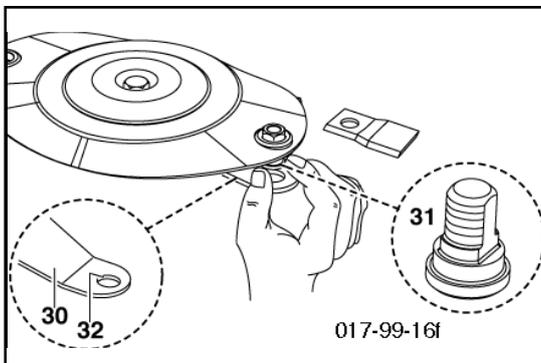
**Checking the mowing blade suspension**
