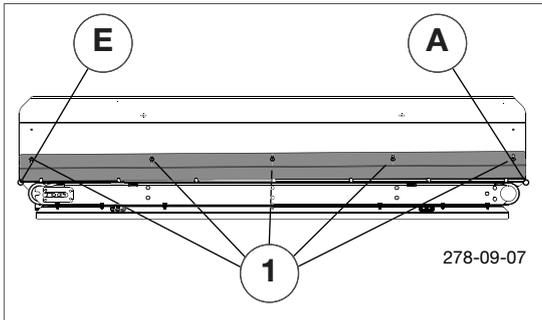
Always set the distance between feed plate and conveyor belt with screws (1) so that gap on conveyor belt ejector side (A) is greater than gap on feed-in side (E). Minimum distance: 5mm
