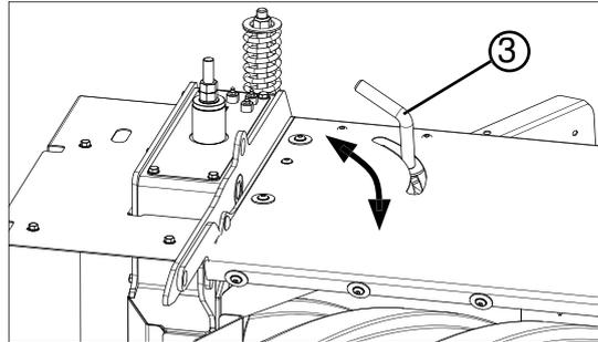
The swath boards shape the cut and conditioned fodder to the desired swath width. Adjusting the swath boards is carried out identically, left and right, by unscrewing and adjusting the setting screw (3)
