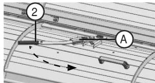
4. Press the lever (2) to the right in order to unlock the lock of the rear wall.
