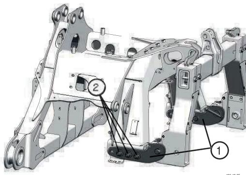
When hitching as Quick Hitch, you must rotate the lower link straps (1) 180°. (see image) balls and spacer sleeves are not used any more.
