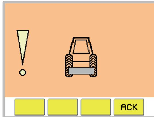
The front mower sensor does not send a response to the job calculator within 6 seconds of pressing the key [Raise front mower] or [Raise all mowing units].
