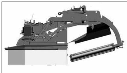
When swinging the rear mower units from transport to working position, the cross conveyors are always to be found in this position (risk of collision).
