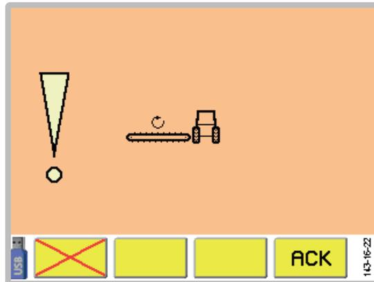
At least one of the cross conveyors is not running, although the cardan shaft is spinning.
