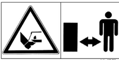
Stay clear of mower knife area as long as tractor engine is running with PTO connected.
