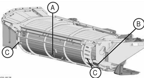
(A)...Middle position for the lever for unlocking the bolts (C)
