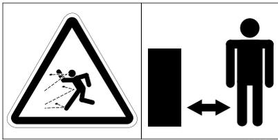
Danger - flying objects; keep safe distance from the machine as long as the engine is running.
