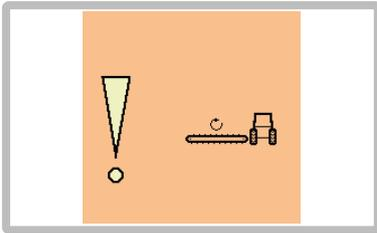
At least one of the cross conveyors is not running, although the drive shaft is.
