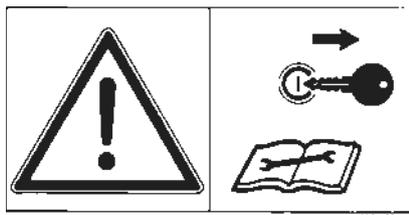
Shut off engine and remove key before performing maintenance or repair work.
