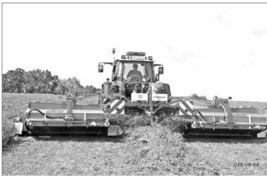
A variable swath deposit is possible using a cross conveyor belt (single swath, broad deposit or triple swath). With the help of the operator terminal, the cross conveyor will be swivelled out or in, and the belt speed per unit infinitely adjusted.
