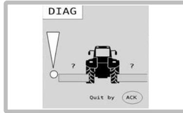
No response from the angle sensors for the rear mower units (B3, B5) .
