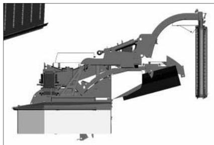
If the swath is not to be manipulated, the cross conveyor belts can be swivelled out.
