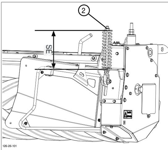
The upper roller is moveable and is tensioned left and right with a spring. The spring preload intensity is set on both sides using the nut (2).
