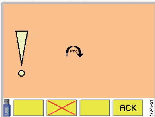
You would like to go into the working position, but the cardan shaft is running.
