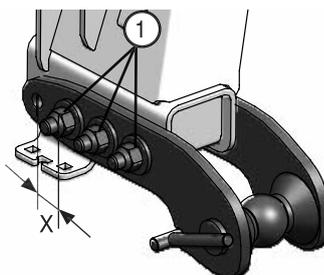
For a possible remedy, shift the two lower link bolts 62.5 mm (X) further from the tractor.
