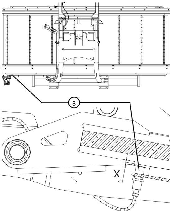
The cross conveyor belt sensor (S) advises the swinging status of the belt. The sensor distance (x) must be configured between 3.5 mm.
