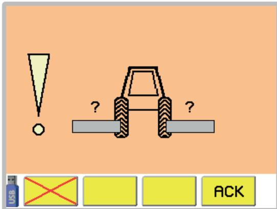
No response from the angle sensors for the rear mower units (B3, B5).
