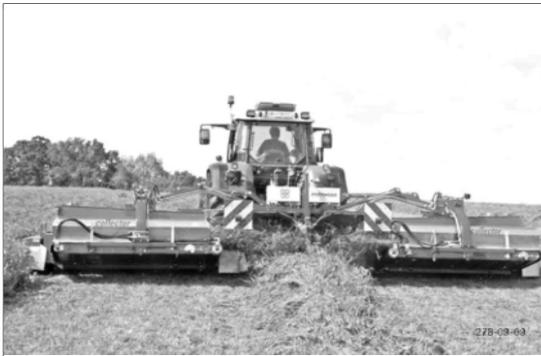
A variable swath deposit is possible using a cross conveyor belt (single swath, broad deposit or triple swath). The cross conveyor is swivelled out or in, and the belt speed per unit infinitely adjusted using the operator terminal.
