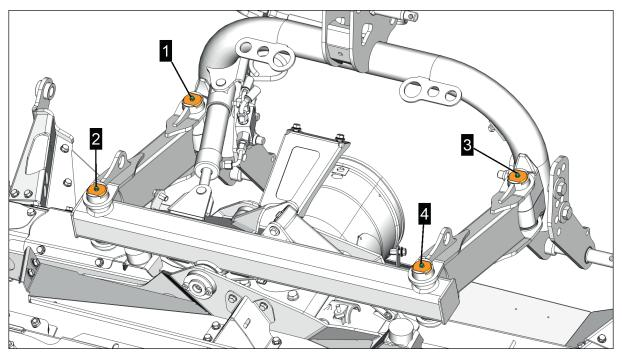
1-4 = Lubricating nipple for cutter bar bearing and lateral shift. Covering blanked out
