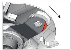
The red marking shows unacceptable traces of wear on one of the mower blade holders. Arrow = Rotation direction during operation.
