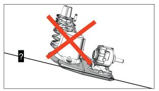
Symbol illustration Horizontally incorrectly aligned!
