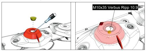
► Loosen M10x35 screw, remove conveyor cones and keep both handy.
