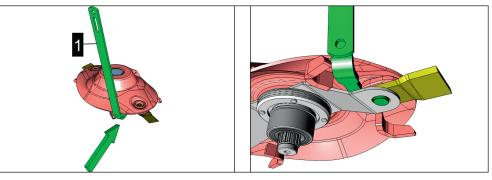
Push the blade wrench down and hold it firmly.The blade holder is also pushed down and the blade is released.
