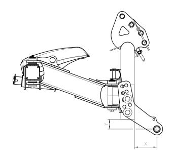
Measurement X = distance from tractor Measurement Y = vertical distance from hitch-on rack
