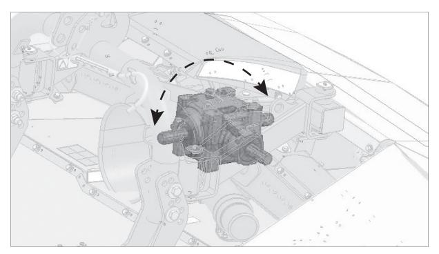
After assembly, restore the correct oil level in the angular gear (for details, see chapter "Maintenance").
