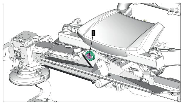
1 = Grease nipple for cutter bar self-aligning bearing
