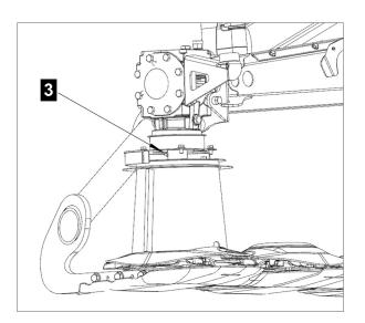
3 = Grease nipple for cardan shaft sliding gear height compensation
