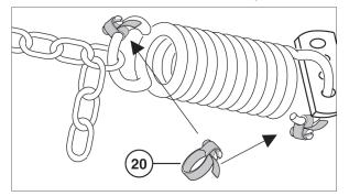
6 The spring tension must be checked whenever the tractor is changed and reset if necessary.
