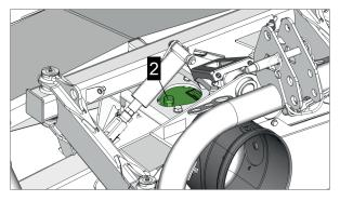
2 = Oil filler plug / oil level measuring rod
