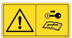
Shut engine off and remove key before carrying out any maintenance or repair work.
