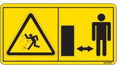
Keep a safe distance as danger exists through parts being ejected while motor is running.
