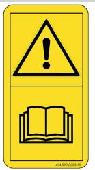
Read the operating manual thoroughly before putting the machine into operation.
