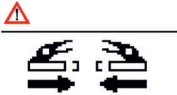
A warning triangle icon is positioned above a horizontal line. Below the line is a diagram showing two side shifters on a machine. Arrows point inward from both shifters, indicating they are being moved to a narrow position.                    | Mettere lo spostamento laterale sulla posizione stretta.                                                                                                                                                       |
