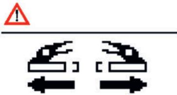
A warning triangle icon is positioned above a horizontal line. Below the line is a diagram showing two side shifters on a machine. Arrows point outward from both shifters, indicating they are being moved to a wide position.                     | Mettere lo spostamento laterale sulla posizione larga.                                                                                                                                                         |
