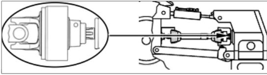
Ensure the proper coverage of the sliding profile in the work and transport position.
