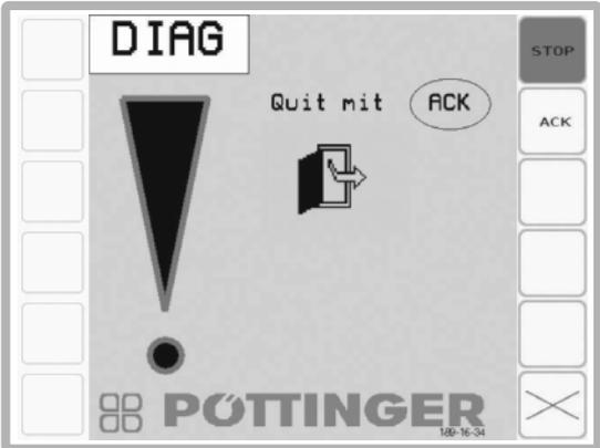
As soon as the climbing aid for the loading area door is unfolded, all hydraulic functions stop, the dosing rollers are uncoupled and the diagnostic notification above appears.
