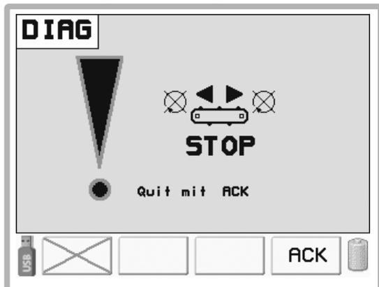
If the cross conveyor belt speed sensor registers no speed 1 second after switching on the cross conveyor, the following error message appears.
