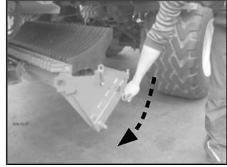
6. Lock the cutter unit with the linchpin (V) in maintenance position.
