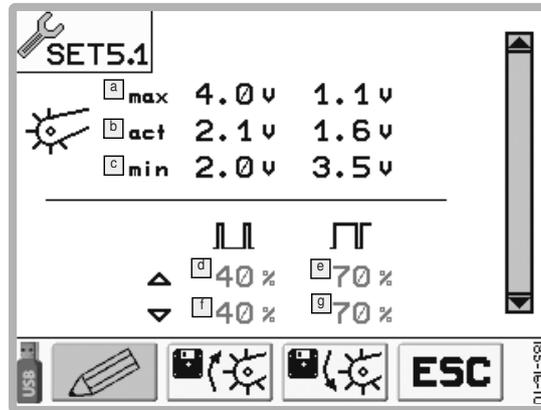
Calibrate the angle sensor
