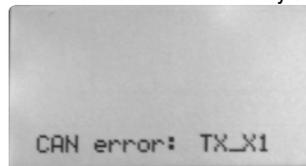
in the figure the connection to module X1 is interrupted
