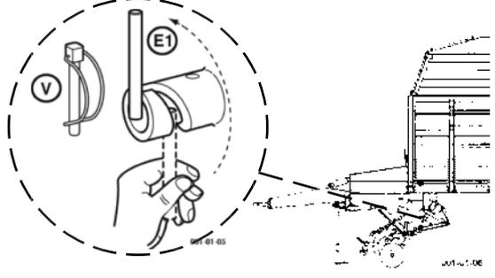
3. Loosen the hydraulic cylinder from the bolt. (right and left side)
