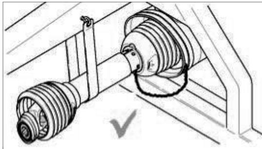
The storage point for the cardan shaft must be located in the front third of the shaft.
