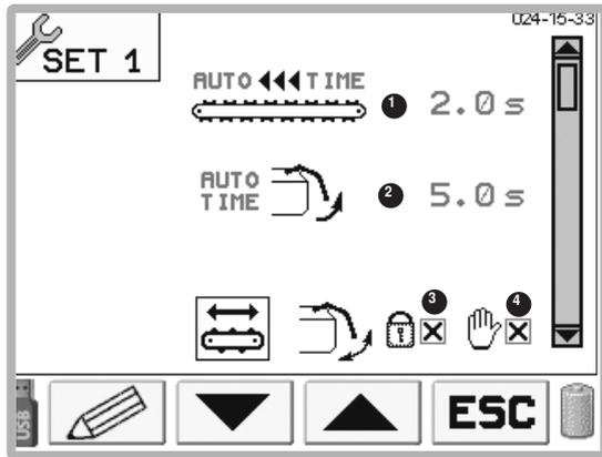
**1** Scraper floor running time for the automatic unloading
