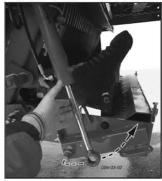
4. Swing the left hydraulic cylinder to the front and lock in the holder (H).
