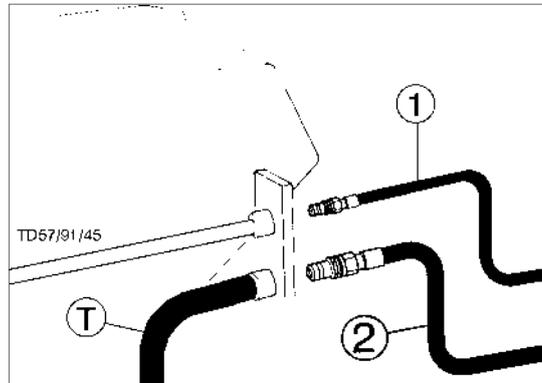
If the tractor is equipped only with single-acting servos, it is absolutely necessary for your specialised workshop to install an oil return pipe (T), if it does not already exist.
