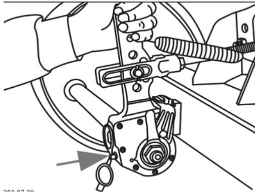
3. Actuate the brake lever repeatedly by hand.
