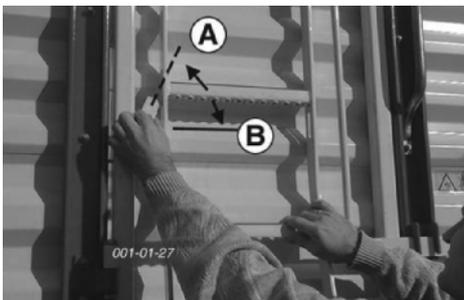
2. The access door in the side wall must only be opened with the drive motor switched off (11).
