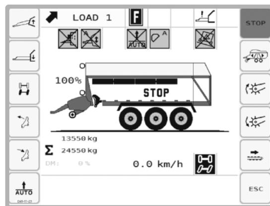
The maximum lock was exceeded. A collision of the tractor's rear wheels with the trailer is imminent. Straighten up!
