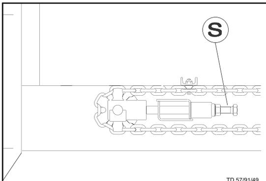
If the tensioning length is no longer sufficient, remove chain links.
