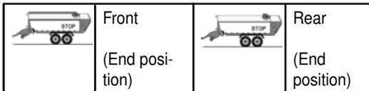
If the load safeguard travels forward or backward, or is located in the midway position, the symbols will blink.
