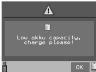
If the battery only has a low residual capacity, the terminal is switched off after 1 minute to avoid exhaustive discharge. (Alarm message in the display)
