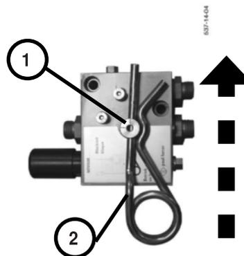
**Emergency brake valve for trailers triggered mechanically**
