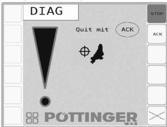
Swivelling the cutting unit in is not possible.
