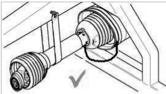
Attach at a straight angle to the cardan shaft, as far as possible.
