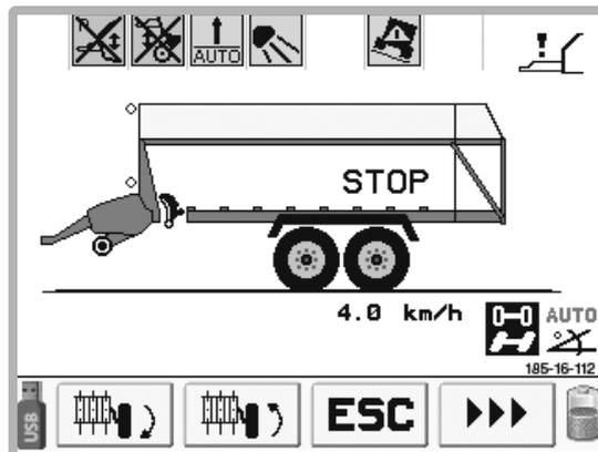
The maximum lock was exceeded. A collision of the tractor's rear wheels with the trailer is imminent. Straighten up!
