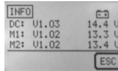
The Info menu provides information on the software version installed and the current voltage
