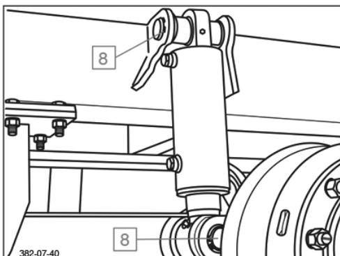
Check damping cylinder mounting for tightness and wear.
