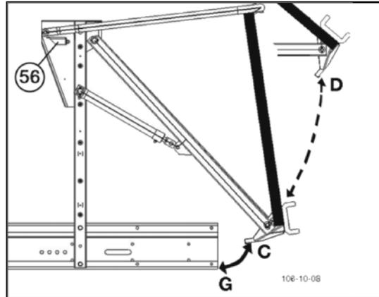
Once in position (C), switch (56) triggers the hydraulic function and the tailgate is closed under pressure (G).
