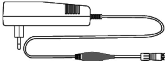
The terminal must be connected at the mains adapter for charging. The mains adapter is to be plugged in at a 230V socket. As soon as voltage is available, the terminal switches on and starts charging regardless of the current capacity. The battery is completely charged and then supplied with trickle voltage. The charging status of the battery is shown in the terminal display.
