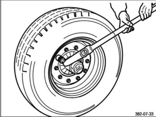
Tighten wheel nuts crosswise with torque wrench.
