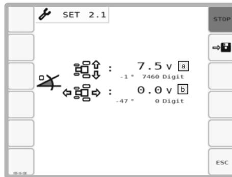
**[a] current value for the lateral inclination**
