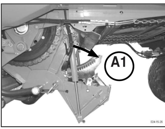
2. Unlock the retaining bolt on the left and right side
