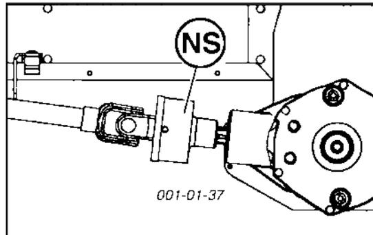
When the discharge beaters are overloaded, e.g. in case of too high scraper floor speed, the shut-off clutch interrupts the torque (= 12 00 Nm).
