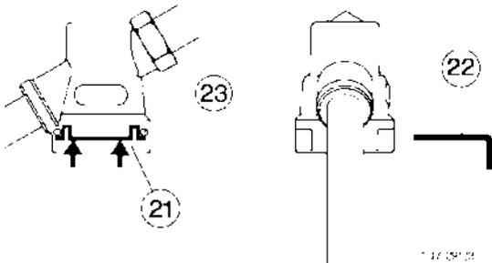
The piston stroke in the brake cylinder may not be greater than 30 mm. Therefore it must be checked from time to time and if necessary readjusted.
