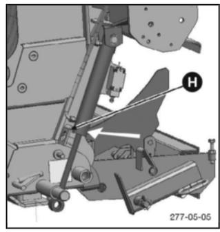
5. Swing out the cutter unit in maintenance position.
