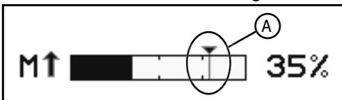
When the pick-up is lowered, the release torque (A) for the scraper floor can be adjusted using the [+] and [-] keys.
