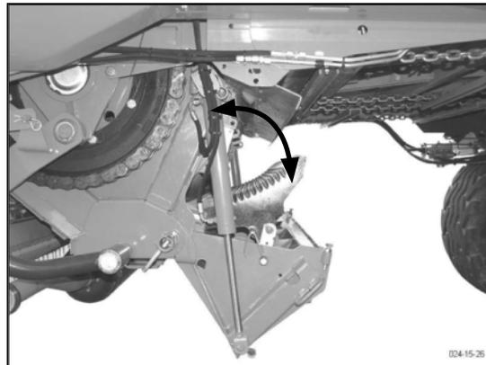
For maintenance work on the cutting unit and the cutter beam, the cutter beam can be swung in or out using both buttons (57).
