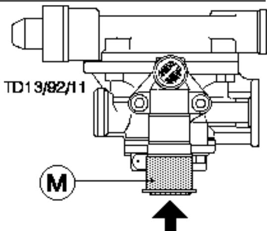
The release position enables wagon to move (shunt) when brake hoses are not connected to the towing vehicle.
