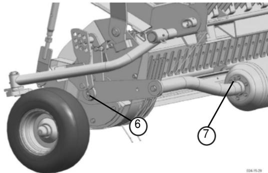
In the sensing roller bearing there is a lubrication nipple (6) on both the left and right sides of the self-loading trailer.
