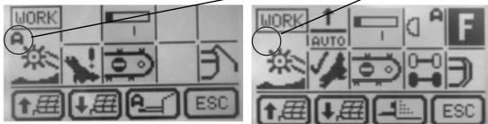
Press shortly the key [Articulated drawbar automatic operation]
