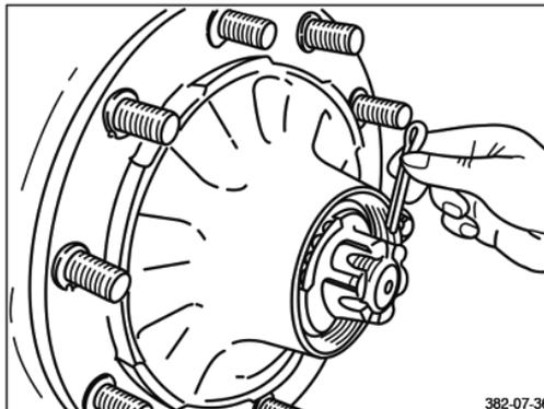
4. Turn crown nut back to the next possible split pin hole. When the holes are identical, return to the next hole (max. 30°).
