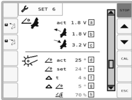
1. Hold the key [Retract cutting unit] pressed until the tension value does not change any more. Then the value for the fully retracted cylinder is saved.
