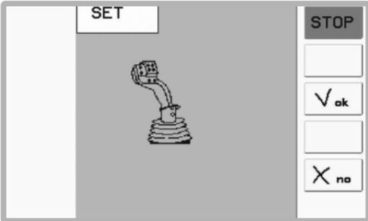
Press the key [ ok ] to release the auxiliary tool. Or press key [ no ] to refuse release and interrupt the operating procedure.
