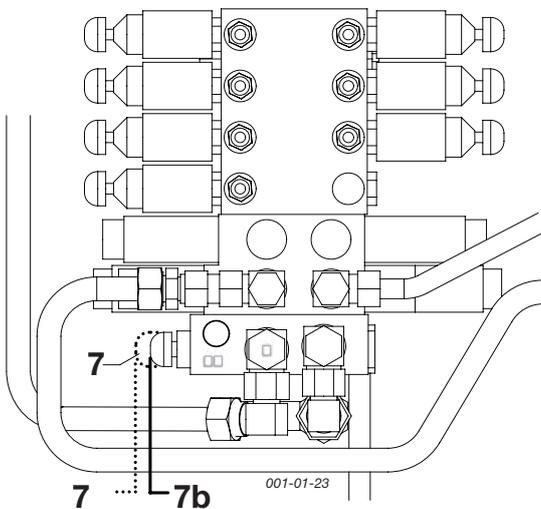
7a Standard position for the open hydraulic system
