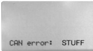
1. Control the bus connection between the operating part and the extension module.
