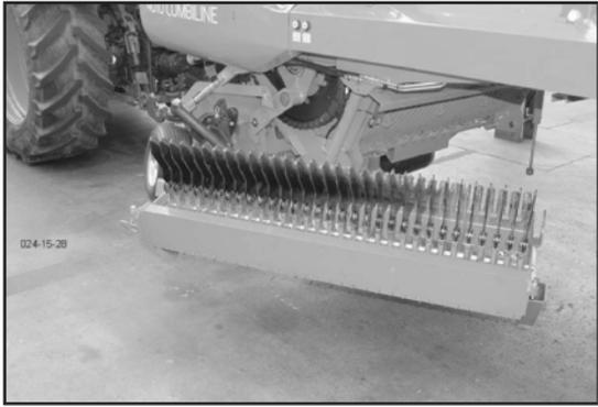
1. Hold down the external button to swing out the cutter beam (A1)
