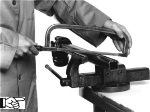
3. Shorten the protective tube by the same length as the corresponding section tube.
