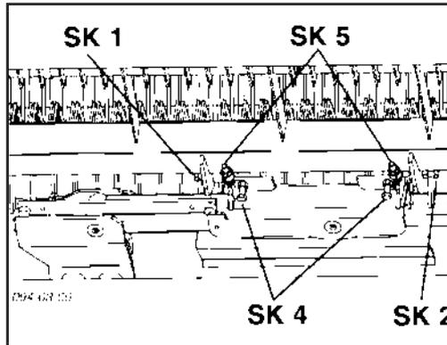
The setting should be so that when the cutter beam is swung back in, the frame tube is able to fit into the opening as closely to the middle as possible (see sketch).
