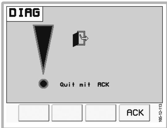
As soon as the climbing aid for the loading area door is unfolded, all hydraulic functions stop, the dosing rollers are uncoupled and the diagnostic notification above appears.
