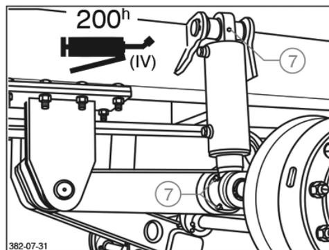
Always make sure that there is no air in the cylinder and the supply line.
