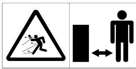
Danger - flying objects; keep safe distance from the machine as long as the engine is running.
