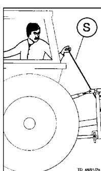
**4. Run stop-lock support release rope (S) into tractor cabin.****5. Set upper link spindle**
