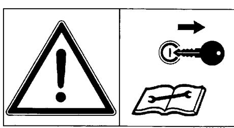
Shut off engine and remove key before performing maintenance or repair work.
