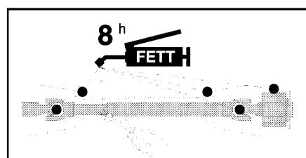
For winter working, grease the tube guards, to avoid them freezing together.
