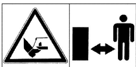
Stay clear of mower knife area as long as tractor engine is running with PTO connected.
