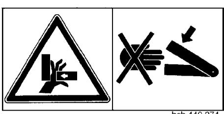
Never reach into the crushing danger area as long as parts may move.
