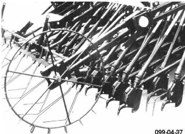
Sowing is driven by a spur wheel, which runs on the surface to be worked. The pressure with which it presses onto the ground may be set by adjusting the spring tension.
