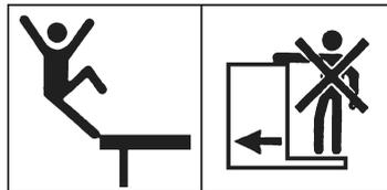
Travelling on implement during operation and transportation is not permitted. Use loading plate or platform only when machine is mounted and standing dormant, or when safely supported.
