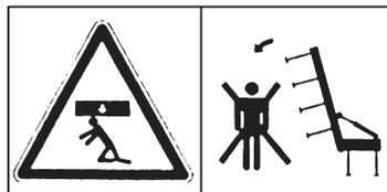
Swivel out side components. Keep your distance. Do not enter swivelling range. Ensure sufficient free space when swivelling out.
