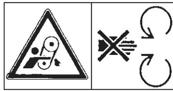
Never open or remove protection devices when drives are running. Keep your distance
