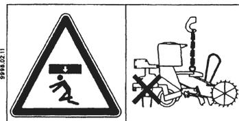
Danger from load above. Lift "Vitasem A" only by transport rings. In the course of this, never lift drill machine together with agricultural implement.
