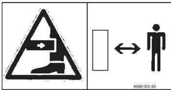
Legs could be hit through components suddenly swivelling out or sliding out. Keep your distance.
