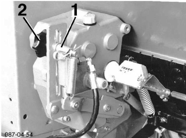
„Normal Amount“ – calibrate as usual; star handle (21/1, page 10) but set as limiter behind the lever (towards 0) – fasten tightly. (Cylinder remains retracted.)
