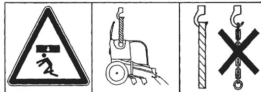
Danger from load above. Lift "Vitasem" in bulkhead wall of seed box. Only use textile belts, no chains.
