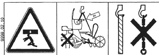
Danger from load above. Lift "Vitasem A" seed box bulkhead wall and transport rings. Use belts. Never lift drill machine together with agricultural implement.
