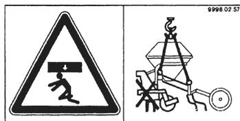
Danger from load above. Lift "Aerosem" only by transport rings. In the course of this, never lift drill machine together with agricultural implement.
