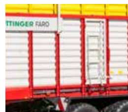
Access door with ladder
