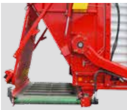
Cross conveyor belt
