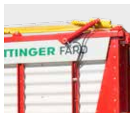
Dry crop extension folds hydraulically
