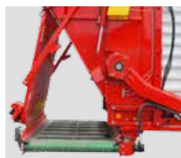
Cross conveyor belt
