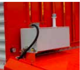
On-board hydraulics for cross conveyor belt
