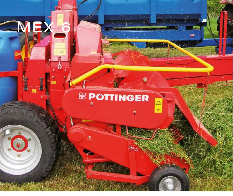
The huge blowing power of the flywheel ensures trailers are filled up right into the furthest corner.
