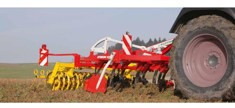
PÖTTINGER SYNKRO cultivators were developed for modern stubble tillages and are suitable for both shallow and deep soil tillage. Particular attention was paid to ease of movement and low power consumption when these machines were designed
