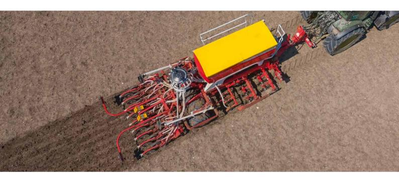
The low draft WAVE DISC with a diameter of 20.08 inch / 510 mm is designed especially for low disturbance drilling. The soil around the WAVE DISC is not moved to the side, but is loosened in strips, thus preventing smearing at seed slot level. Row spacings of or 4.92 or 6.57 inch / 125 or 167 mm are available. A row spacing of 6.57 inch / 167 mm is recommended for regions with extremely heavy, wet and sticky soil conditions. The WAVE DISC is available for all TERRASEM mulch seed drills.
