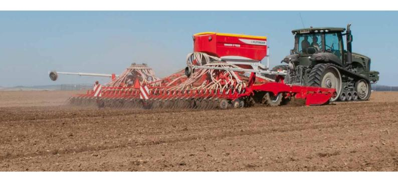
The TERRASEM mulch sowing concept from PÖTTINGER combines soil tillage, recompacting and sowing in a single machine. The effective compact disc harrow, the unique tire packer and the perfect coulter rail ensure optimum results.
