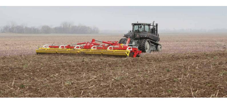
The TERRADISC compact disc harrow was developed for stubble breakage and general seedbed preparation. The compact design and aggressive disc position ensure reliable forage and good mixing of harvest residues.
