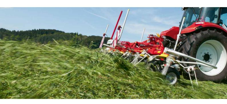
Our tried and tested tedders offer perfect contour following. This allows you to ted the crop in a way that is gentle on the forage without introducing dirt. The wide wheels, in conjunction with the MULTITAST wheel on the headstock, significantly improve slope capability. The high quality of workmanship guarantees a long service life.
