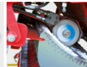
AUTOCUT on-board knife sharpening
