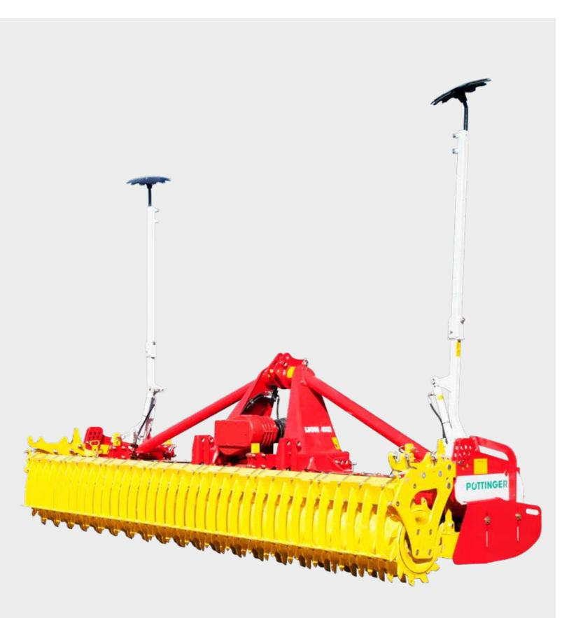
These professional machines have working widths of 3.0 and 4.0 m and are equipped with advanced technology to handle all soil conditions. You can rely on this LION in the most demanding situations.
