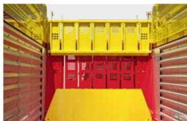
The automatic loading system guarantees that the wagon is filled to achieve maximum transport capacity. The forage is already carefully compressed in the transfer throat to make full use of the loading chamber.
