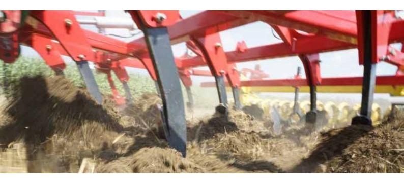
The PÖTTINGER SYNKRO cultivators have been developed to deliver optimum stubble cultivation and are suitable for both shallow and deep tillage. During the design phase, special attention was paid to low drag resistance and low power requirement.
