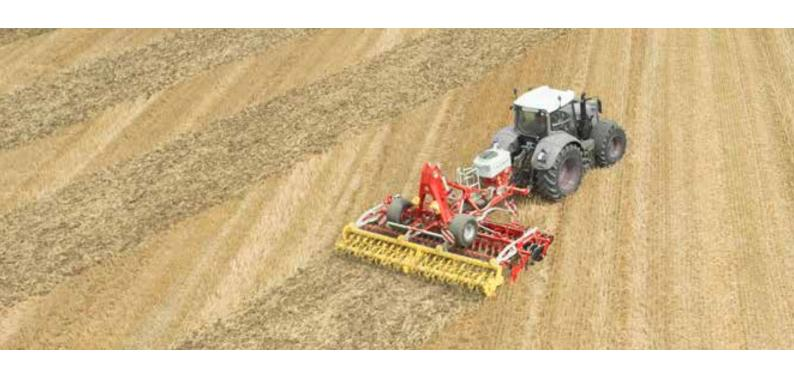
The TEGOSEM cover crop sowing unit combines soil cultivation and sowing a catch crop in a single pass to save time and costs. The TEGOSEM can be combined with LION power harrows, FOX compact combinations, TERRADISC disc harrows as well as with SYNKRO stubble cultivators. This seed drill can be used together with three-point mounted implements and trailed machines.
