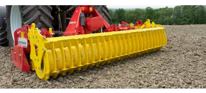
Intensive crumbling for the best quality tilth and excellent mixing of the soil are the highlights of PÖTTINGER power harrows. Combined with a PÖTTINGER seed drill, this machine becomes a high output and cost effective combination delivering perfect drilling results.
