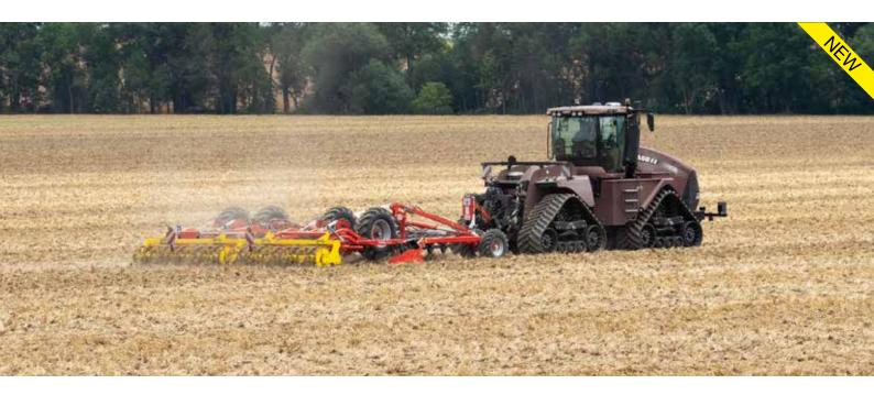
TERRIA trailed machines cover a wide range of applications in soil cultivation. Perfect ground tracking is a prerequisite for working at the same depth across the whole working width, every square metre of soil is valuable. Fully versatile to meet the highest expectations.
