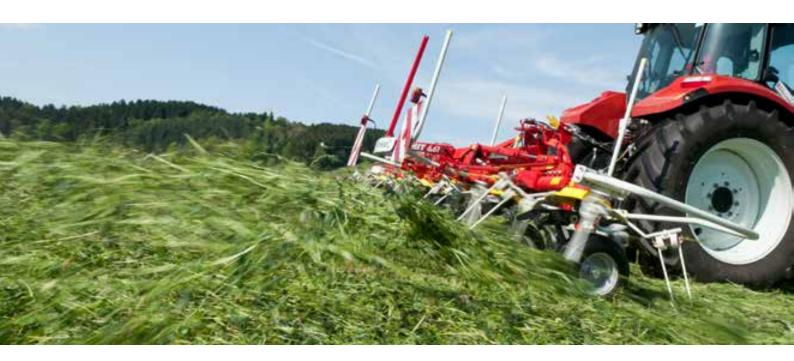
Our proven rotary tedders deliver perfect ground tracking. Tedding crops carefully without dirt ingress is the result. The wide wheels together with the MULTITAST jockey wheel on the headstock greatly improve performance on slopes. High manufacturing quality guarantees a long service life.
