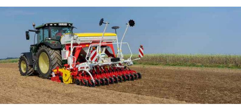
The unique AEROSEM seed drill concept from PÖTTINGER unites the drilling of cereals and maize. Precision universal metering and perfect coulter systems guarantee exact placement of the seed.
