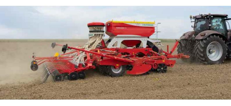
The maintenance-free WAVE DISCs have a diameter of 510 mm and are available with row spacings of 12.5 cm or 16.7 cm. The working depth is infinitely-variable controlled by a hydraulic system like on all TERRASEM drills. The PÖTTINGER WAVE DISC system is ideal for difficult soil conditions that require reduced tillage. The WAVE DISC is available for all TERRASEM mulch seed drills.
