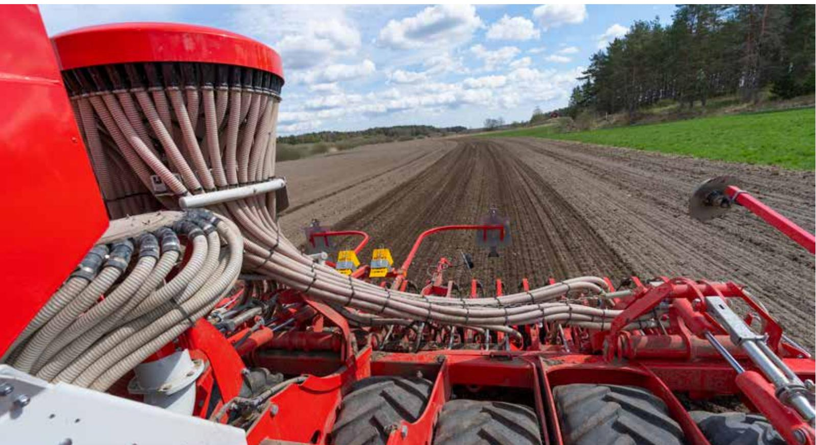
The proven tyre packer provides the necessary consolidation ahead of the coulters to create perfect germination conditions for the seed. Consolidation is necessary because the soil has been loosened many times and needs to be connected to the moist subsoil in order to ensure the capillary action needed for water to reach the seed and provide the level of moisture required for germination.
