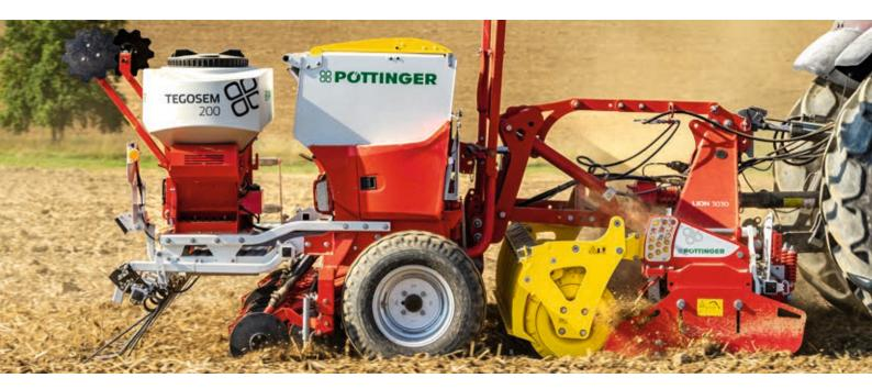
When the TEGOSEM is combined with seed drills and soil preparation implements, two processes can be carried out in a single pass. This is a fast and cost-effective way of sowing a cover crop or similar material at up to 40 kg/ha. As a result, it opens up a number of different capabilities with different machine combinations.
