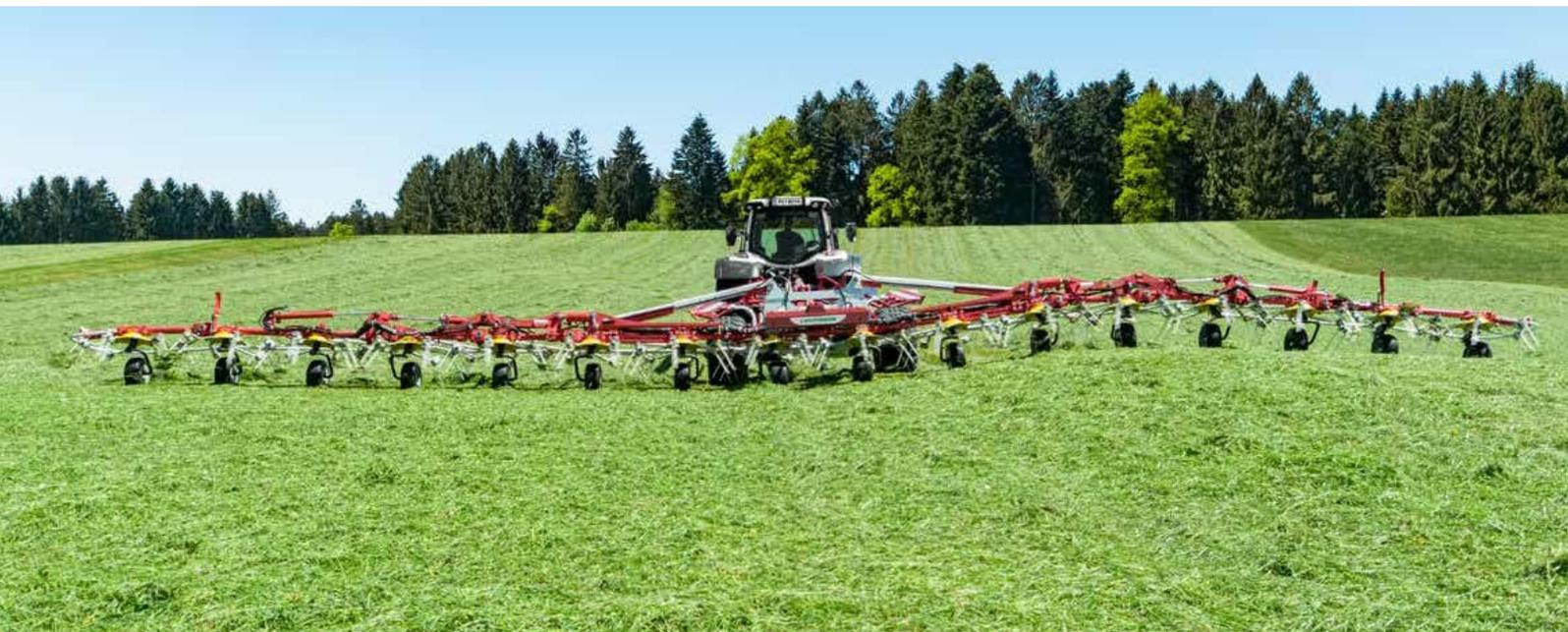
Our proven rotary tedders deliver perfect ground tracking. Both the mounted and trailed tedders feature jockey wheels located close to the tine arc to react to any bumps. In addition, all frame joints follow every contour independently of one another. The tines do not touch the ground. Tedding crops carefully without contamination entering the forage is the result.
