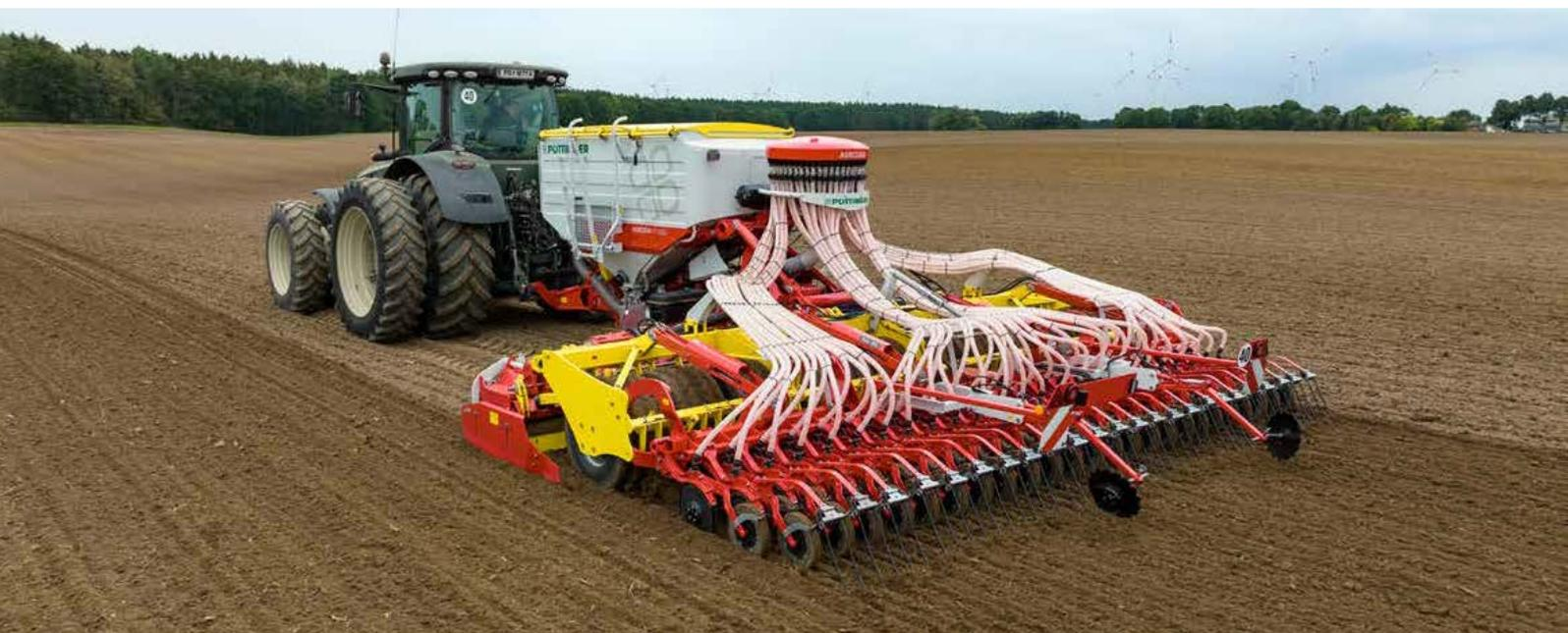
The trailed AEROSEM seed drill combination with active tillage combines seedbed preparation with a LION power harrow, consolidation with a grooved tyre packer and sowing with the DUAL DISC coulters. The trailed seed drill concept has been developed for light to the heaviest soil types and enhanced with the profiline comfort control system. This lets you control all the hydraulic functions, including coulters pressure adjustment, conveniently from the tractor cab.
