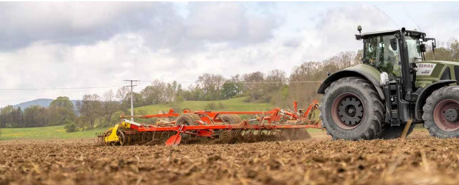
Regardless of whether its stubble cultivation and weed control, incorporating cover crops or seedbed preparation, the trailed PLANO shallow cultivator is the specialist in soil water conservation and mechanical weed control thanks to its shallow, full-surface slicing action. Medium-depth tillage down to 15 cm is also possible for a high output, cost-effective and energy-efficient application.
