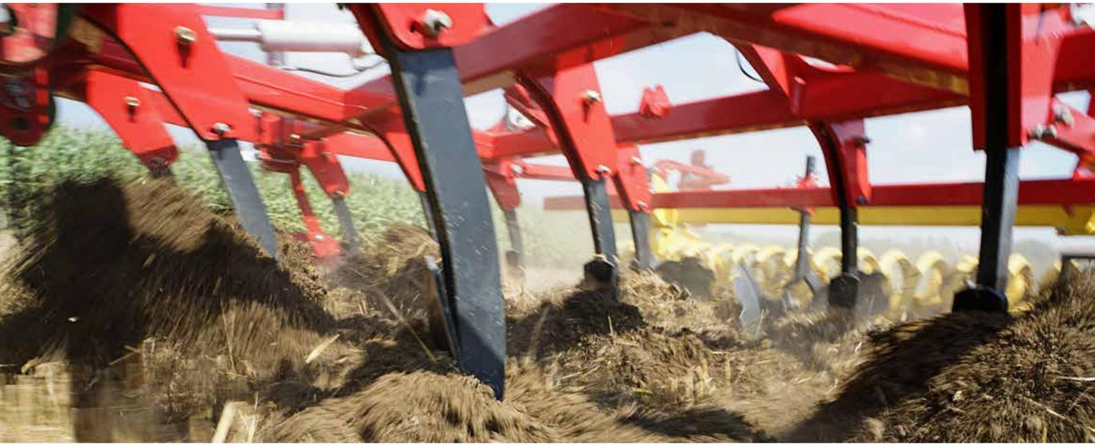
The PÖTTINGER SYNKRO stubble cultivators have been developed to deliver optimum stubble cultivation, and are suitable for both shallow and deep tillage. During the design phase, special value was placed on reducing draft and power requirements.
