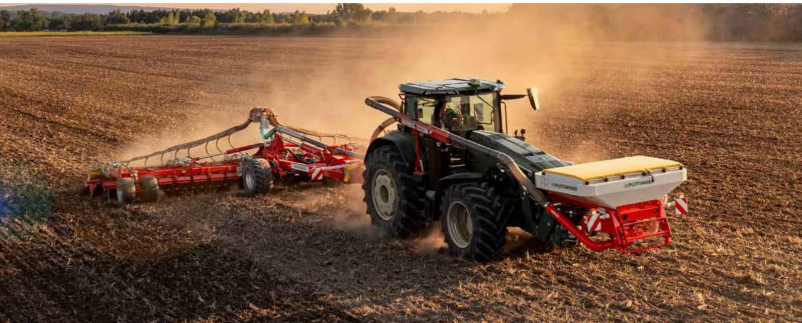
The AMICO F hopper in combination with various arable machines offer the possibility to apply fertiliser or microgranules, cover crops or two components, at the same time. With capacities of 1,700 and 2,400 litres and a division of 60:40, a wide range of applications is guaranteed.
