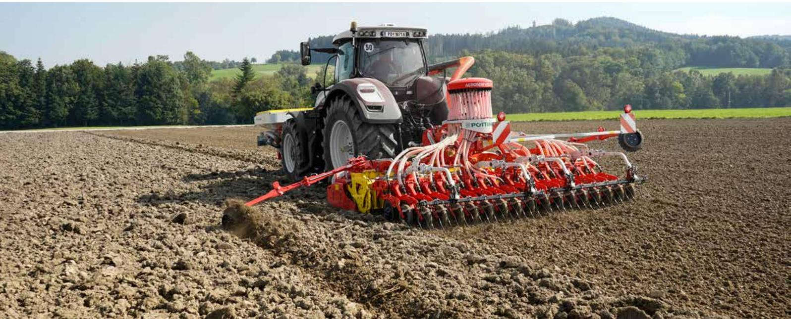
The AROSEM F front hopper seed drill extends PÖTTINGER's range of pneumatic implement-mounted seed drills up to a working width of 6 metres.
