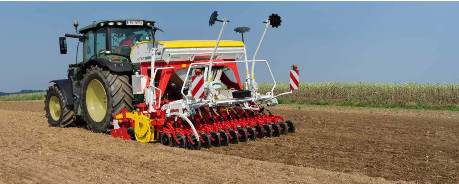
The unique AEROSEM seed drill concept unites the drilling of cereals and maize. Precision universal metering and coulter systems proven time and again in the field guarantee exact placement of the seed.
