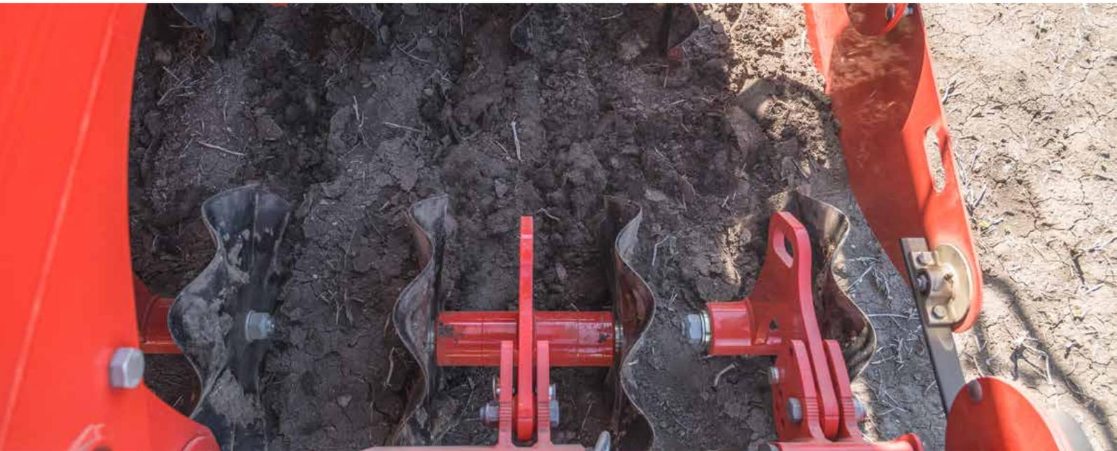
The maintenance-free WAVE DISCs have a diameter of 510 mm and are available with row spacings of 12.5 cm or 16.7 cm. The working depth is infinitely-variable using a hydraulic system. The PÖTTINGER WAVE DISC system is ideal for difficult soil conditions that require reduced tillage. The WAVE DISC is available for all TERRASEM universal seed drill combinations.
