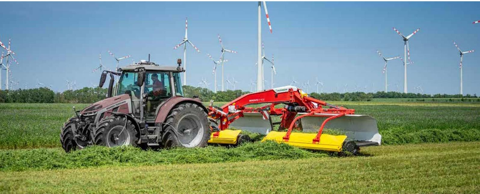
MERGENTO collects the forage from the ground using the pick-up. Without further contact with the ground, cross conveyor belts transport the forage to the swath. Dirt and stones remain on the ground. Disintegration losses are reduced to a minimum.
