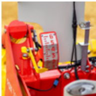
Hydraulic working depth adjustment
