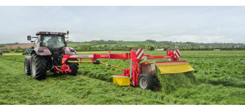
Our NOVACAT T trailed mowers with a working width of 9'11" / 11'4" are ideal for mowing with small tractors. On the trailed version with chassis, you do not need any lifting power, so you can also use lower power tractors. This helps you save fuel.
