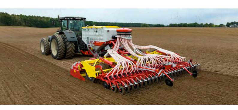
The trailed AEROSEM seed drill combination with active tillage combines seedbed preparation with a LION power harrow, consolidation with a grooved tyre packer and sowing with the DUAL DISC coulter rail. The trailed seed drill concept has been developed for light to the heaviest soil types and enhanced with the profiline comfort control system. This lets you control all the hydraulic functions, including coulter pressure adjustment, conveniently from the tractor cab.
