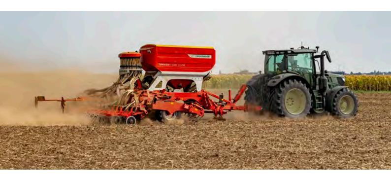
The TERRASEM V CLASSIC models without tillage tools offer smooth running and high output technology for covering large areas. When using these seed drills, the seedbed has already been optimally levelled in advance. Perfect seed placement in a consolidated seedbed is achieved thanks to the optimum ground tracking of the coulter rail and the unique tyre packer.
