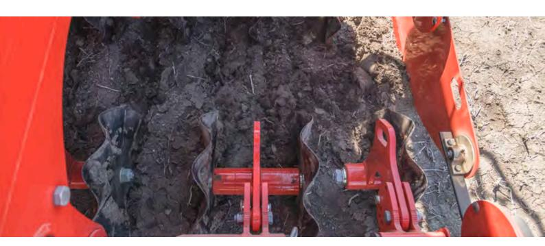
The maintenance-free WAVE DISCs have a diameter of 510 mm and are available with row spacings of 12.5 cm or 16.7 cm. The working depth is infinitely-variable using a hydraulic system. The PÖTTINGER WAVE DISC system is ideal for difficult soil conditions that require reduced tillage. The WAVE DISC is available for all TERRASEM universal seed drill combinations.
