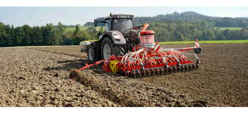
The AEROSEM F front hopper seed drill extends the range of PÖTTINGER pneumatic implement-mounted seed drills with a working width of 3 m to 6 m.
