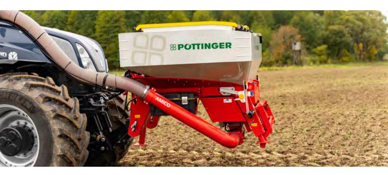
The AMICO F hopper enables a wide range of applications. Up to 2400 litre capacity and two metering units offer full flexibility and high output. Combined with various tillage machines, two work steps can be combined to save precious time.
