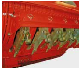
Bolt-on frame with 6 / 11 knives
