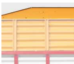
Crop deflector board for steel superstructure
