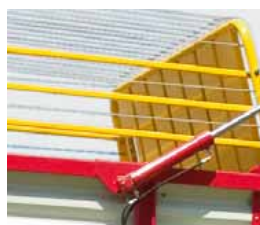
Dry crop extension folds hydraulically
