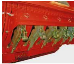
Bolt-on frame with 6 / 11 knives
