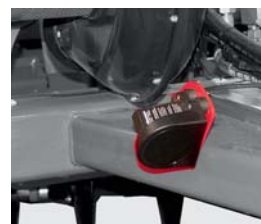
Radar sensor for metering system
