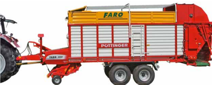
D wagon – version with beaters (3rd beater and cross-conveyor optional)
