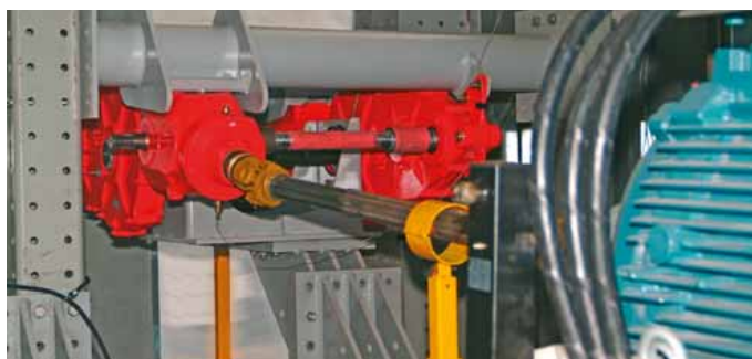
The performance of the drive elements is tested in the transmission test.
