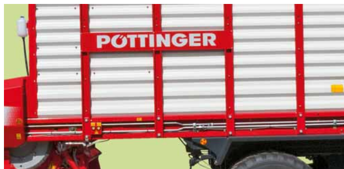
Profile panels with special coating – close spacing of side columns
