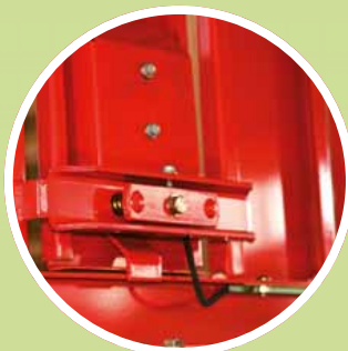
❶ Sensor on the front gate
