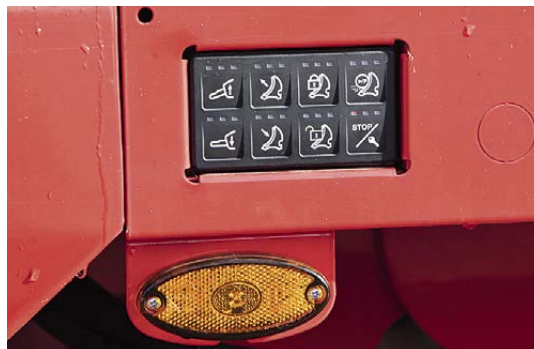
The new operator control unit controls various functions through the Can-Bus, a boon for attachment/removal and for grinding and swapping knives.
