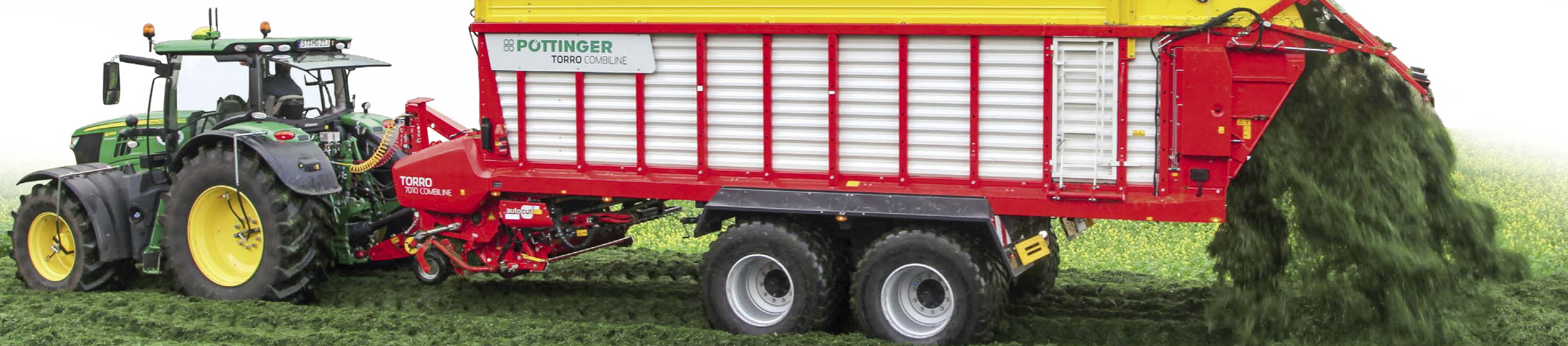
The discharge gearbox can now handle 200hp, which is enough to clear out wet grass in less than 1.5 minutes! Photos: Wilmer
