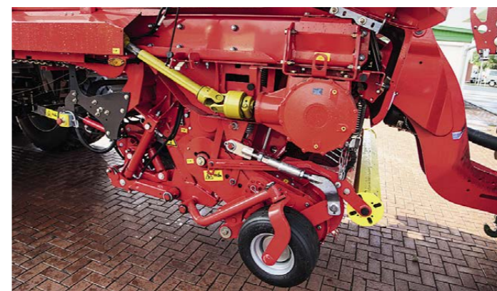
The pto shaft for the discharge beaters runs down the right hand side of the machine and is now overload protected by a 1,700Nm clutch.
