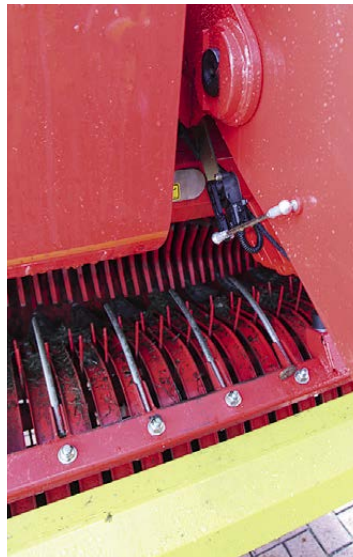
New sensors everywhere - the speed and inclination sensors (bottom) control the auto-lock function of the caster steer axle. The torque sensor (far left) forms part of the automatic loading system. The angle sensor (left) controls the articulated drawbar.
