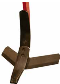
Hardened chisel points and armoured goose foot shares
