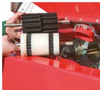
Easy change between coarse and fine metering wheels
