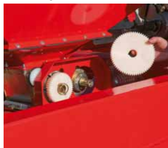
Drive gears are easily interchanged
