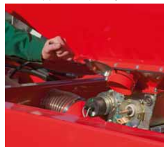
Outlet slide to empty the seed hopper completely
