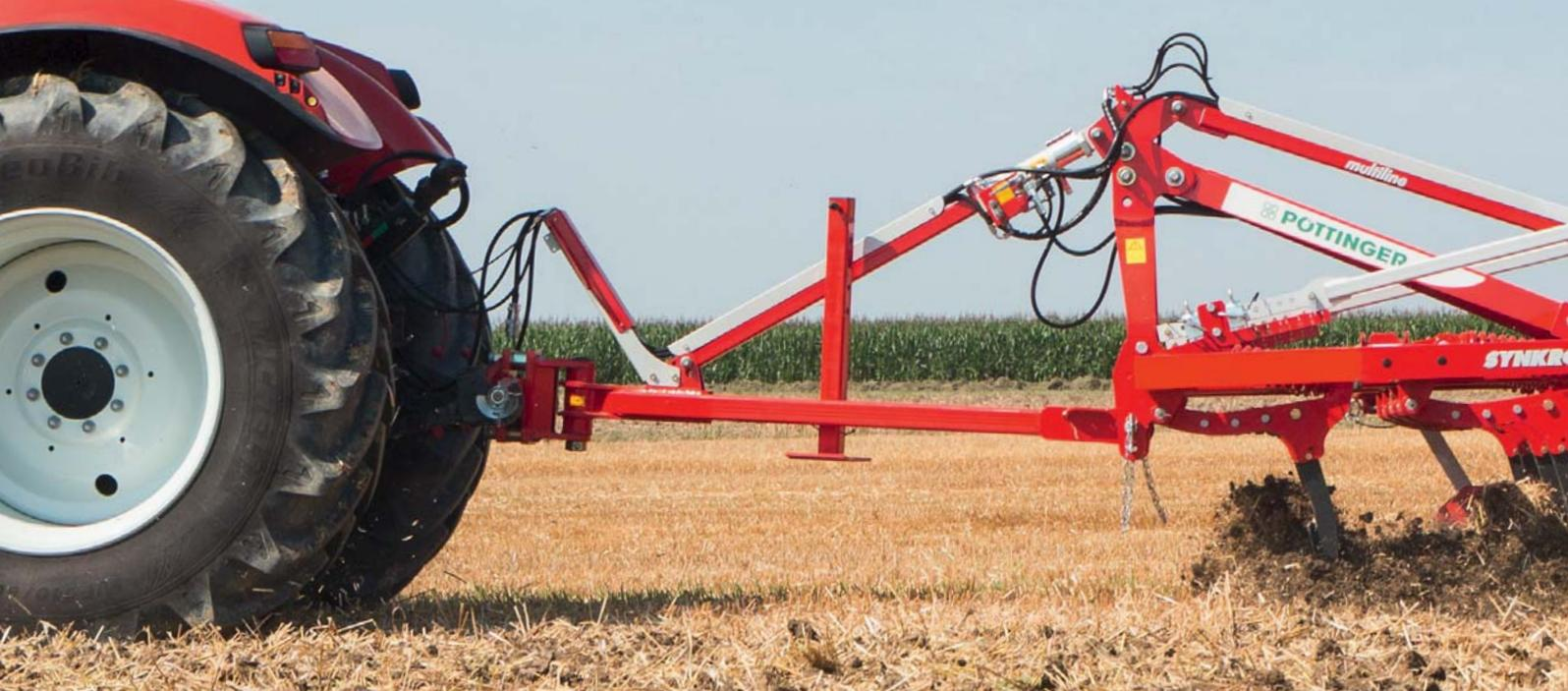
**The implement-mounted VITASEM can be used flexibly in combination with TERRADISC disc harrows or SYNKRO stubble cultivators, a LION power harrow or FOX compact combination. Moreover, the TERRADISC and SYNKRO can also be used on their own for soil cultivation.**
