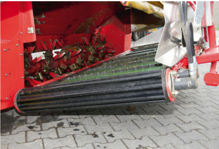
The test mower carried an optional accelerator roller at the inboard end of each belt. Like the belts, these are powered by the unit's own hydraulic pack.
