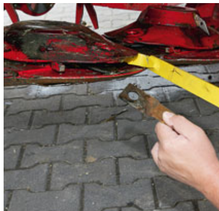
Novacat mowers are established units. Blade changes are simple and won't be needed so often now that tougher blades are standard.
