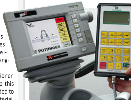
Pöttinger's Power Control box (right) is a minimum specification requirement. If you opt to handle mower function through the tractor's ISObus unit (left), then Power Control's functions include an area meter.
