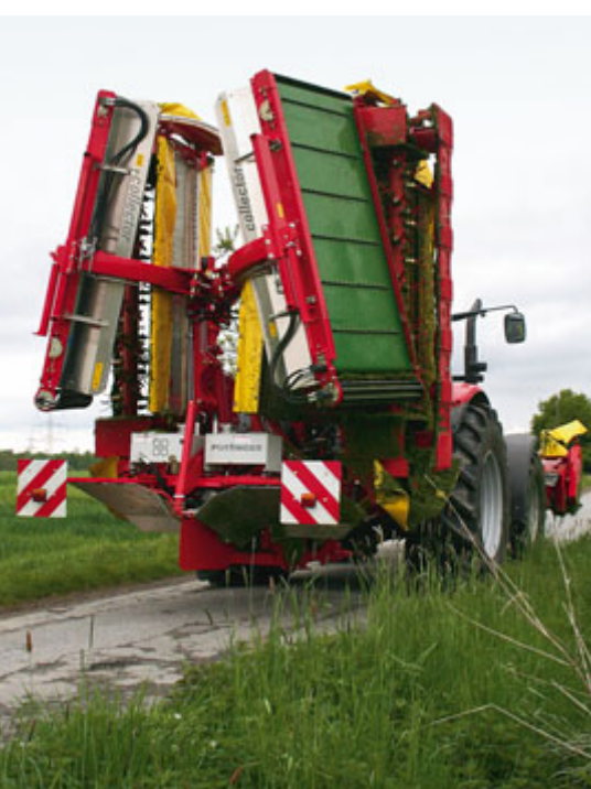
The rear mowers and Collector weigh in at 3.61t; the front unit adds 1.18t. On some 200hp tractors that might be too much.
