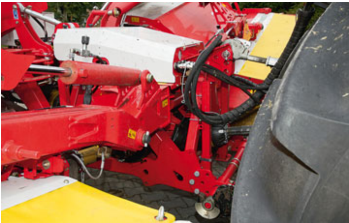
The headstock looks suitably stout. That's good, as the Collector adds another 1.18t. Depending on the tractor and tyres, the unit's lower link pick-up points might need to be repositioned forward.
