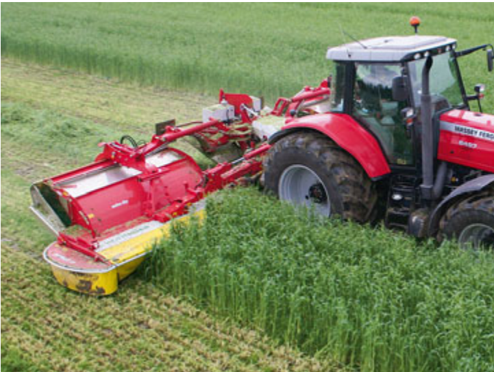
The test mower controlled bed pressure hydraulically. The Collector rides on coil springs.
